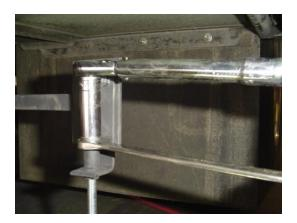
15. Double check the Mini-skirt heights and tighten the upper 5/16" nuts together on both sides. Torque to 9 ft. pounds.
