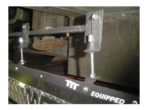
10. Attach the mini-skirt to the lower bracket per drawing 1. Ideally the bottom of the miniskirt will hang 3 1/8" above the ground. There are 3 places to adjust the height of the mini-skirt. The top / bottom bracket interface, the mini-skirt mounting plates, and fine adjustment is on the 5/16" x 4" hex bolts.
