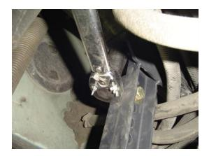
8. Place a 3/8" nut plate on the top of the frame rail aligning the nuts to the new holes. Hold the top bracket up to the bottom of the frame rail and bolt on using (2) 3/8" x 1 1/2" hex bolts, and (2) 3/8" flat washers. Torque bolts to 45 ft. pounds.
