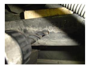
7. Check for wires / hoses prior to drilling and move or protect with a wooden block. Using a 13/32" drill bit and the clamped top bracket as a guide, drill 2 holes though the bottom of the frame rail. Note: It is easier to mark the center of the holes with a 3/8" bit, remove the bracket, then drill though with a 3/16" followed by the 13/32" drill bit.
