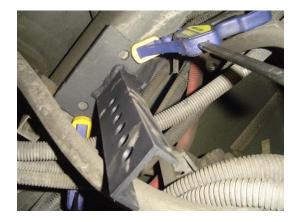
4. Once a suitable location has been determined clamp the bracket to the bottom of the frame rail. The flat side of the channel should face the outside of the coach and the flat side of the angle should align with the inside edge of the frame rail.
