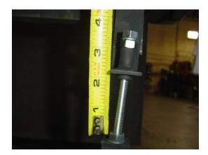
11. Use these positions to adjust the height of the mini-skirt. Allow for  $1 \frac{1}{2}$  travel of the 4" bolt on the hanger.
