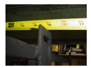
6. Make final adjustments to the position of the top bracket now, using the lower bracket as a place to measure from. Ideally the mini-skirt mounting plates should be 15" back from the tire mud flap, or 17" from the tire, and the top bracket aligned with the inside edge of the frame rail.
