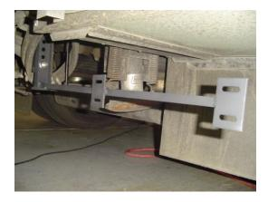
5. Bolt the bottom bracket to the top bracket using (2) 1/2" x 1 1/2" hex bolts, (2) 7/16" flat washers, and (2) 1/2" flange nuts. The bolts should be located as far from each other as possible. Finger tighten. The bottom bracket should hang as close to the bottom of the compartment as possible with the mini-skirt mounting plates toward the rear of the coach.
