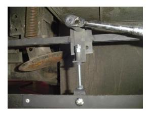
16. Bounce the Mini-skirts up and down a few times on the 4" bolts to align the inside hangers, ensure the 4" bolts are straight down, then tighten the inner top 5/16" nuts to the bracket. Torque to 9 ft. pounds.
